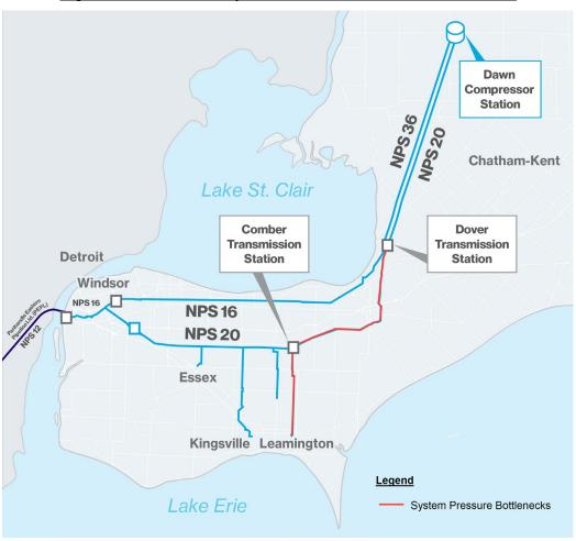
Figure 4: Panhandle System Current Pressure Bottlenecks
