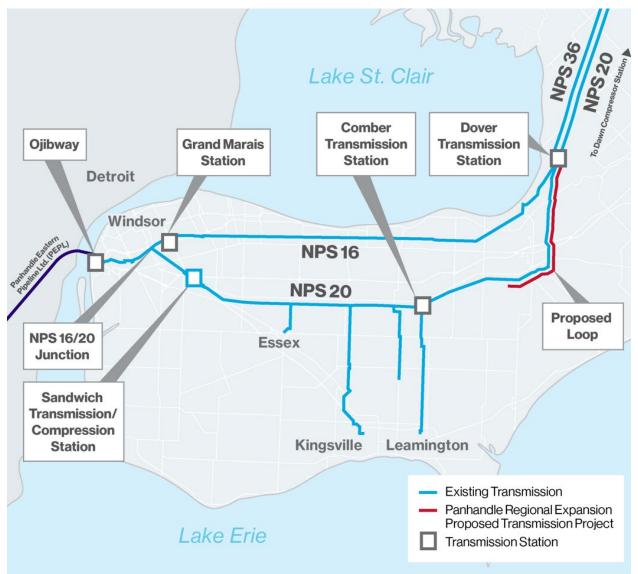
4. The Project will commence at the existing Enbridge Gas Dover Transmission Station located 40 km southwest of the Dawn Hub at Balmoral Line and Town Line Road in Chatham-Kent, Ontario. The pipeline will loop the existing NPS 20 Panhandle Line, following existing easements where possible, for approximately 19 km to Richardson /U
