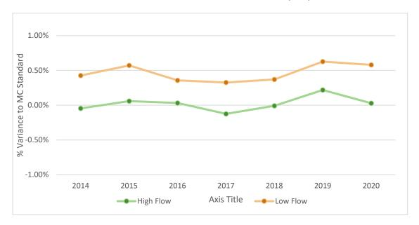
Figure 6: LUG Meter Test Results vs Measurement Canada (MC) Standard
