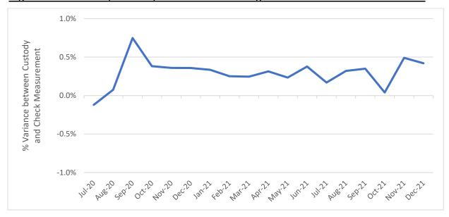
21. In 2022, Enbridge Gas installed a new Measurement Canada certified remote terminal unit (RTU) at the Gatineau interconnect, which ensured that both custody and check measurement is in place, whereas only one source of measurement was previously available. This also enabled an increased level of data validation by the team accountable for gate station measurement.
