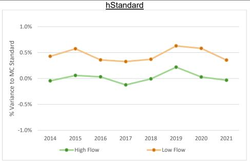
Figure 5: Union Rate Zone Meter Test Results vs Measurement Canada (MC)
