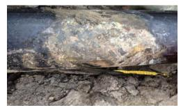
Figure 5.2-26: Coating damages
