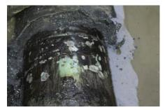
Figure 5.2-24: Multiple corrosion sites on NPS 12 St. Laurent pipe
