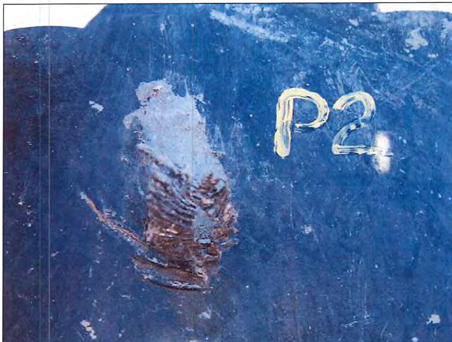
Photograph 19 • Site 2. Sample of Coating Damage by Locating Probe (P2).
