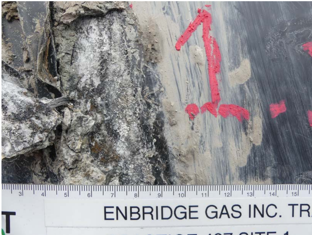
021 - CD-01 COATING REMOVED, CLOSE UP OF CORROSION DEPOSIT
