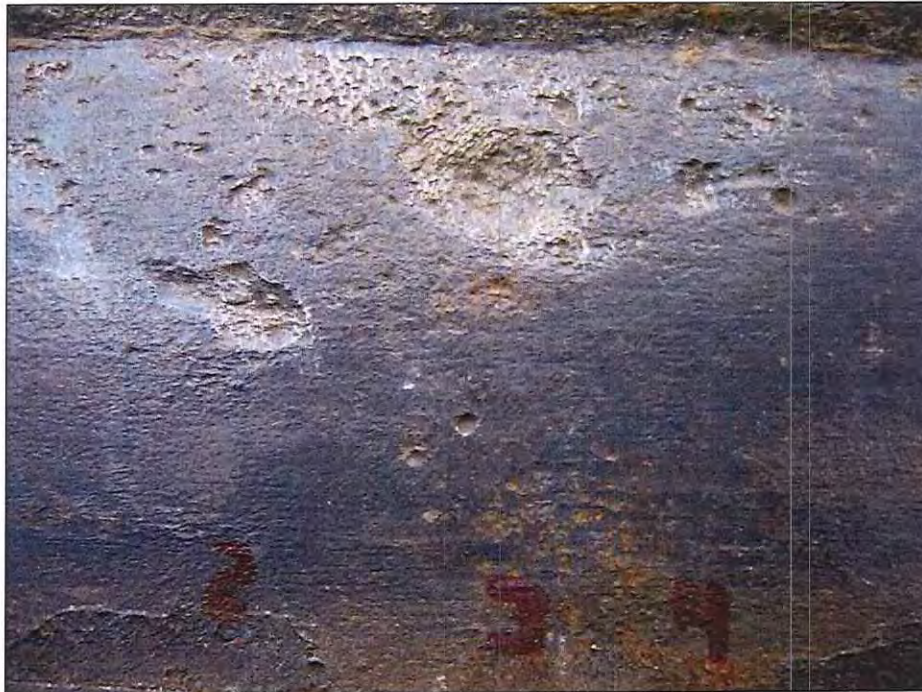
Photograph 25 • Site 2. Sample of Shallow Pits (R12 – Pit #'s 2, 3 & 4).
