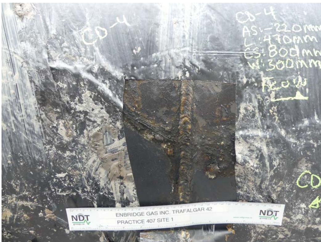
036 - CD-04 COATING REMOVED, BLACK, ORANGE CORROSION DEPOSITS
