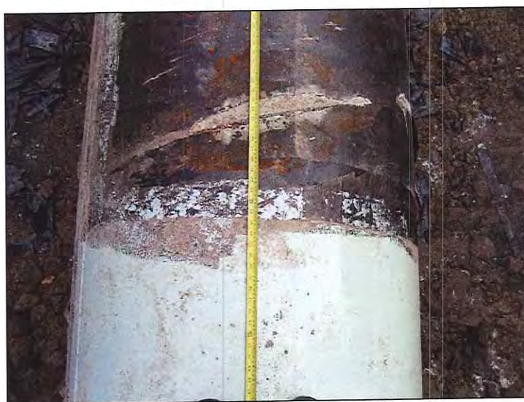
Photograph 5-9 • Site #1. Pipe Exposed. Corrosion at Overlaps
