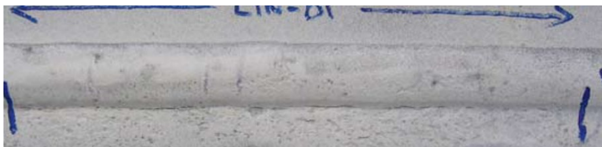
Figure 7: Typical Trafalgar NPS 42 Dawn to Kirkwall Toe Cracking SCC (2020)
