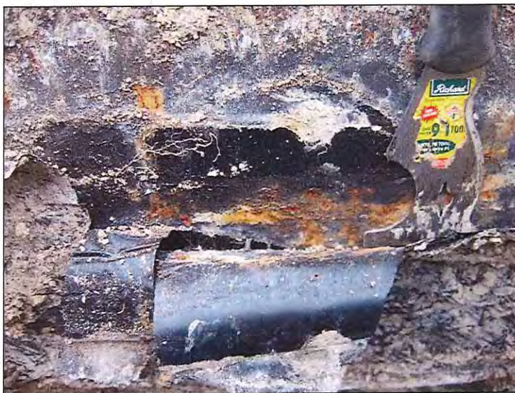
Photograph 5-4 • Site #1. Sample of Coating Damage. Ch. 69.45m (640cm)
