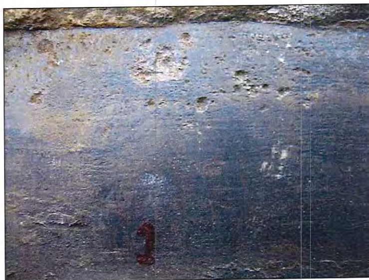
Photograph 5-25 • Site #2. Sample of Shallow Pit (R12-Pit #1)
