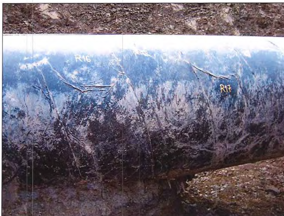
Photograph 12 • Site 2. Disbonded Coating at Longitudinal Weld. Looking South – 02.
