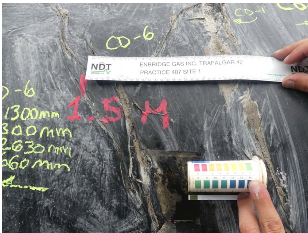
041 - CD-06 COATING REMOVED, ELECTROLYTE PH TAKEN
