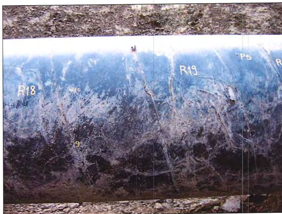
Photograph 14 • Site 2. Disbonded Coating at Longitudinal Weld. Looking South – 04.
