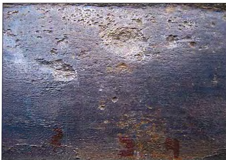
Photograph 5-26 • Site #2. Sample of Shallow Pits (R12-Pit #'s 2, 3 & 4)
