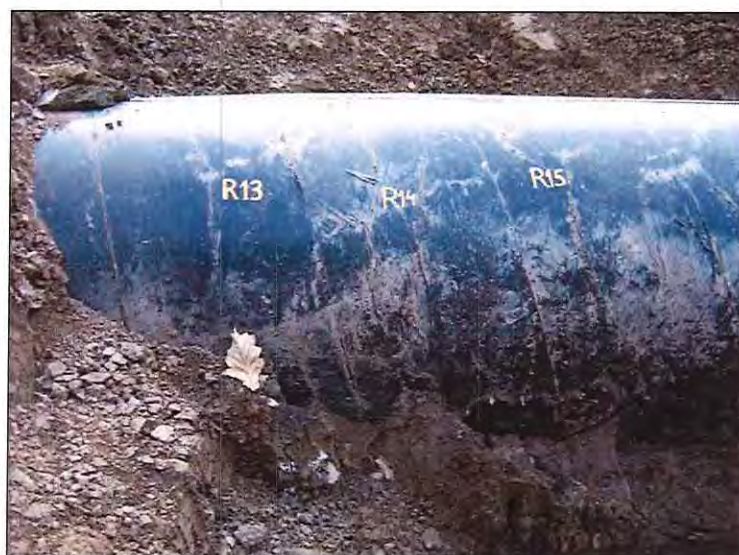
Photograph 5-19 • Site #2. Sample of Disbonded Coating along Longitudinal Weld. Looking South
