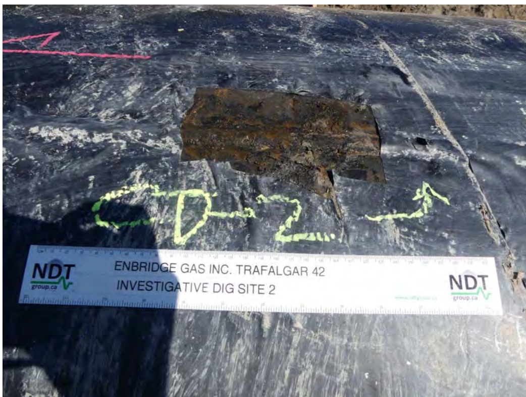
020 - CD-02 COATING REMOVED BLACK CORROSION DEPOSIT
