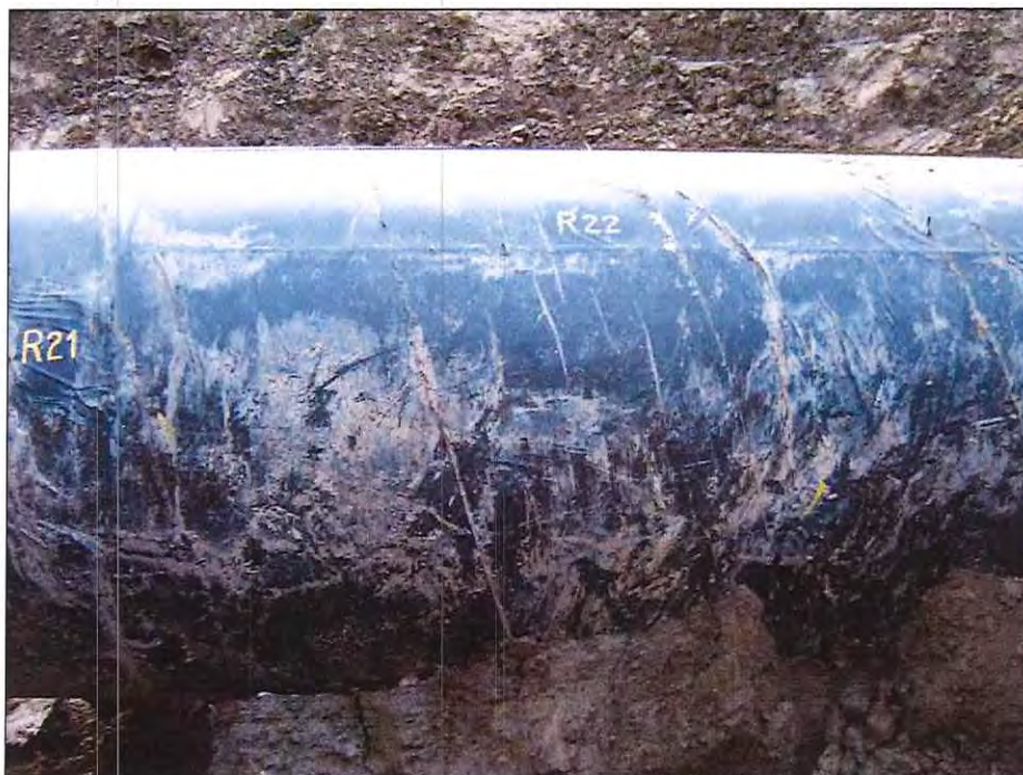
Photograph 16 • Site 2. Disbonded Coating at Longitudinal Weld. Looking South – 06.
