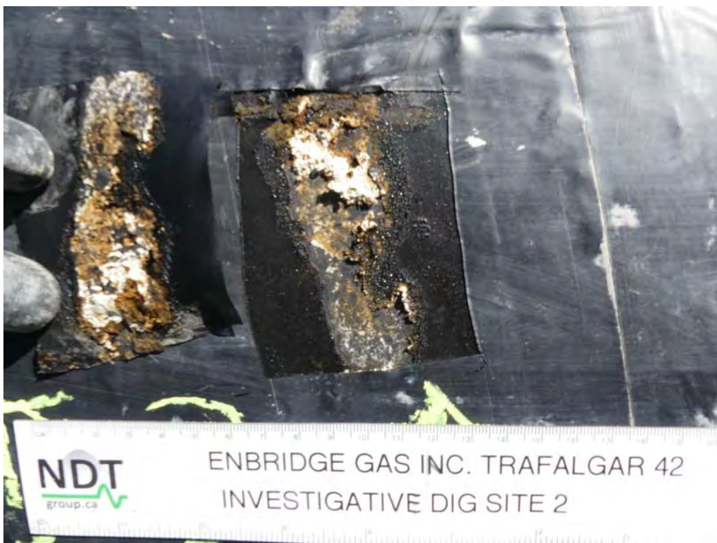
030 - CD-03 COATING REMOVED WHITE, BLACK CORROSION DEPOSIT (2)
