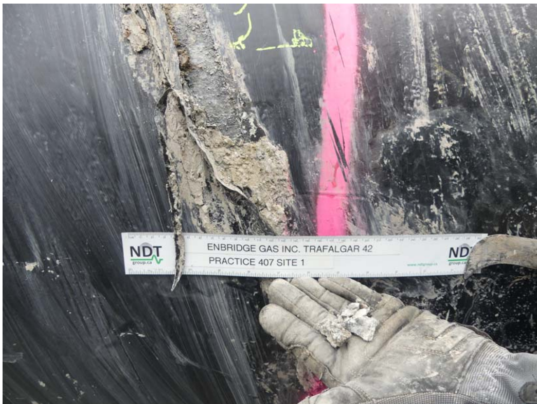
022 - CD-01 COATING REMOVED, WHITE HARD CORROSION DEPOSIT
