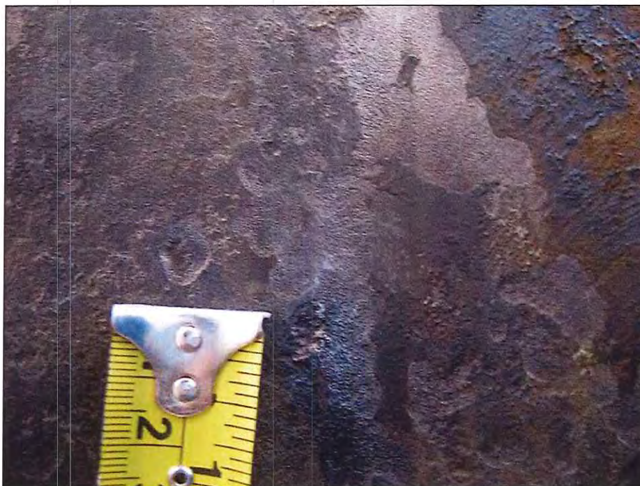
Photograph 11 • Site 1. Pit Cluster #1. Ch. 70.10m (7.05m). Close View.
