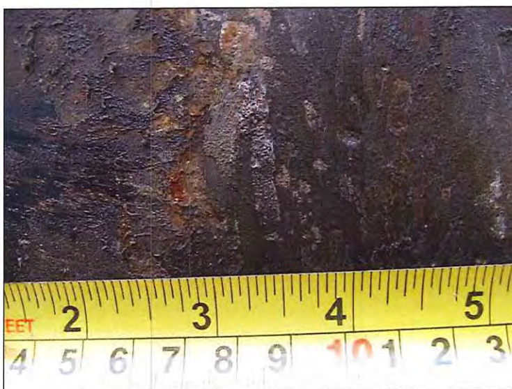
Photograph 5-15 • Site #1. Pit Cluster #3. Ch. 67.65m (4.6m). Close View
