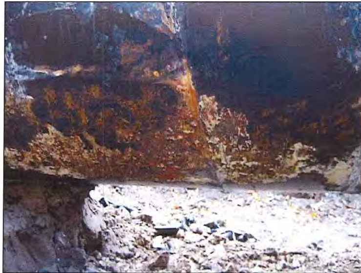
Photograph 5-7 • Site #1. Pipe Exposed. General Corrosion & Calcareous Deposits
