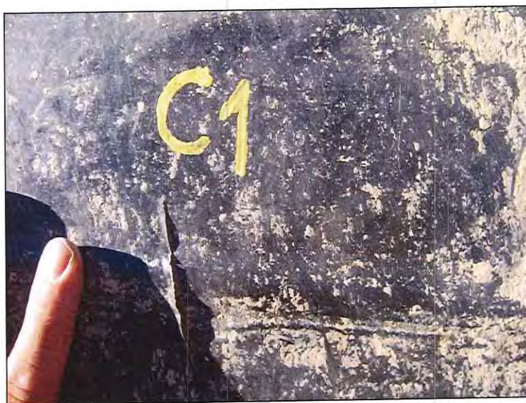
Photograph 5-21 • Site #2. Coating Damage. Sample of Coating Cut (C1)
