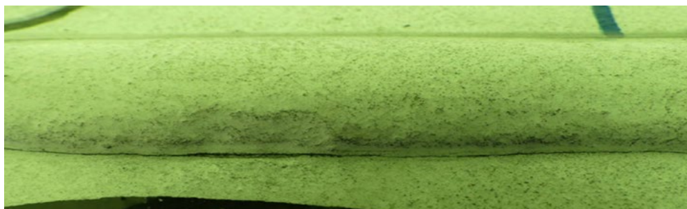
Figure 6: NPS 42 Dawn to Cuthbert Toe Cracking SCC (2019)
