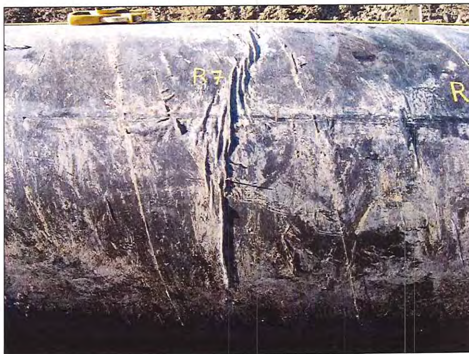
Photograph 6 • Site 2. Disbonded Coating at Longitudinal Weld. Looking North – 04.
