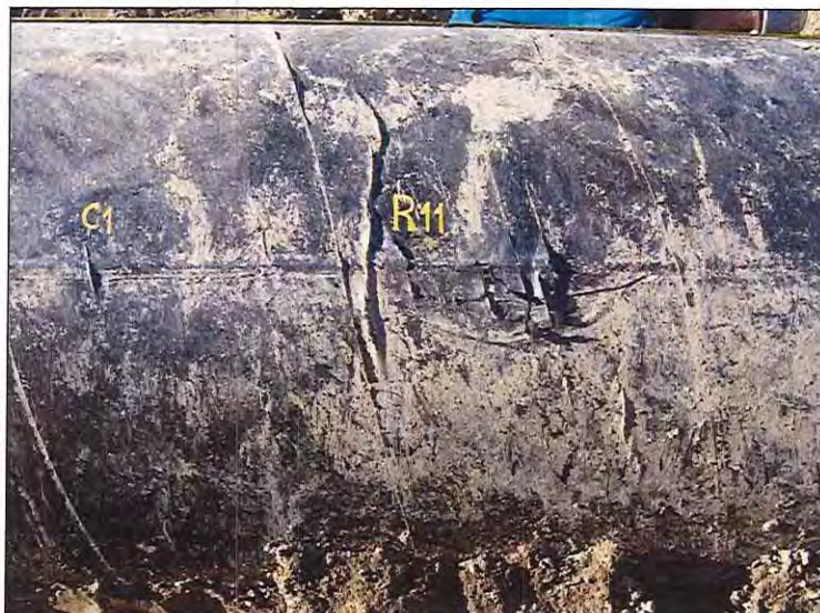
Photograph 5-18 • Site #2. Sample of Disbonded Coating along Longitudinal Weld. Looking North
