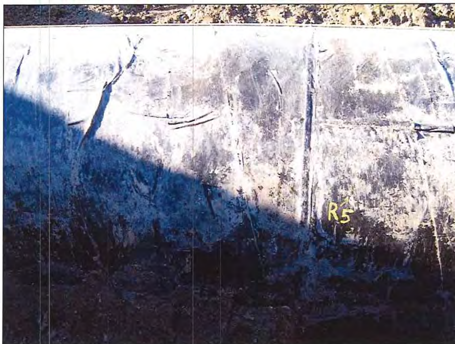
Photograph 8 • Site 2. Disbonded Coating at Longitudinal Weld. Looking North – 06.
