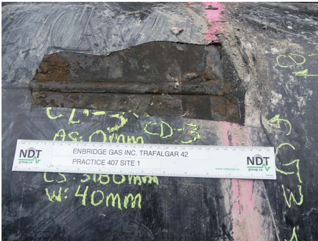
033 - CD-3 COATING REMOVED, BLACK, ORANGE COATING DEPOSITS
