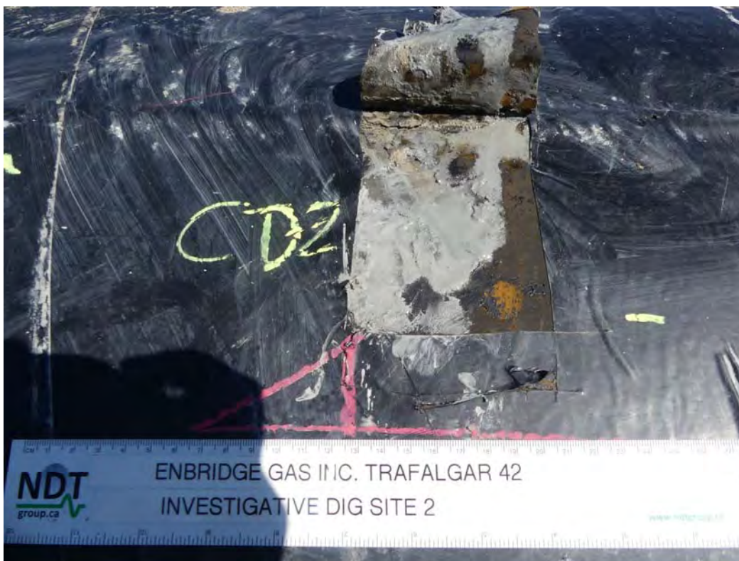
022 - CD-02 COATING REMOVED PASTY GREY CORROSION DEPOSIT CLOSE-UP
