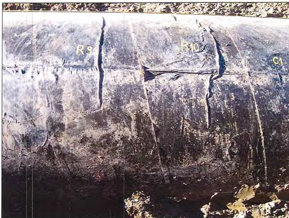
Photograph 4 • Site 2. Disbonded Coating at Longitudinal Weld. Looking North – 02.
