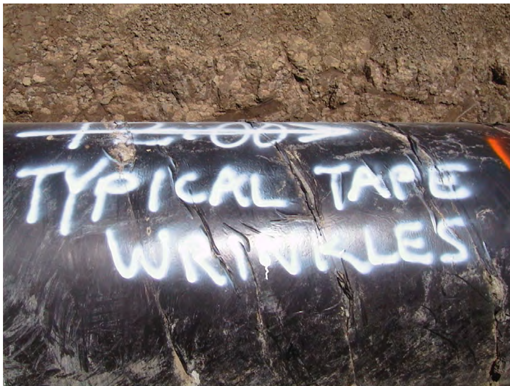
Photo showing typical tape wrinkles along entire dig site
