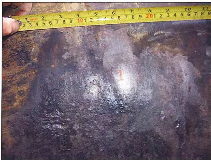
Photograph 5-10 • Site #1. Pit Cluster #1. Ch. 70.1m (7.05m)
