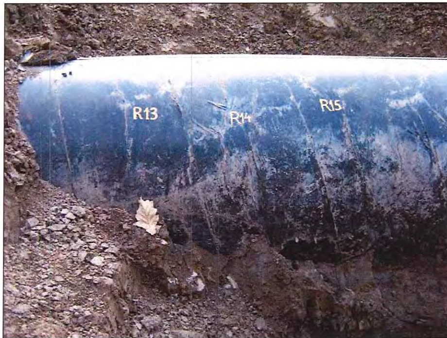
Photograph 11 • Site 2. Disbonded Coating at Longitudinal Weld. Looking South – 01 (East).
