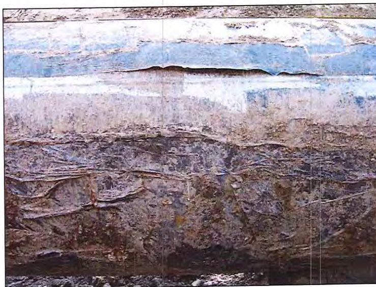
Photograph 5-6 • Site #1. Wrinkled Coating. Looking South
