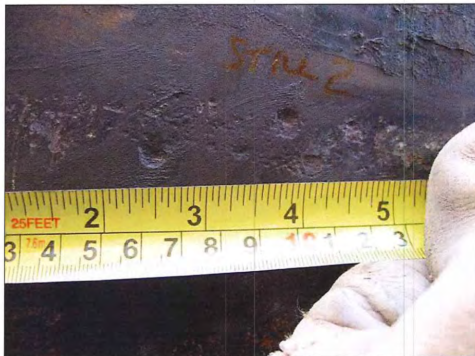
Photograph 13 • Site 1. Pit Cluster #2. Ch. 69.45m (6.40m). Close View.
