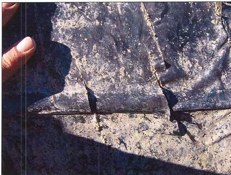
Photograph 20 • Site 2. Coating Damage. Sample of Disbonded Coating (R5).
