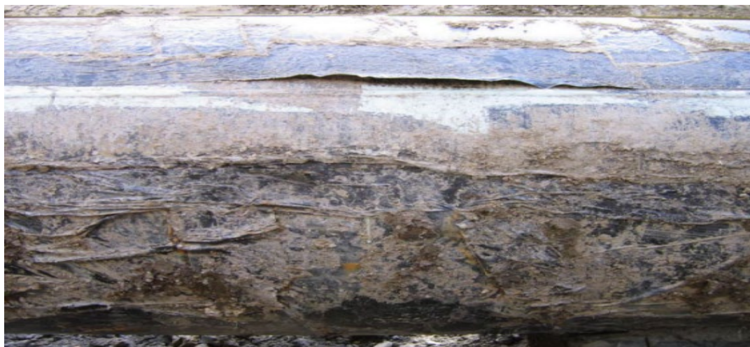
Figure 4: NPS 42 Dawn to Cuthbert Disbonded Polyken Tape Coating (2005)
