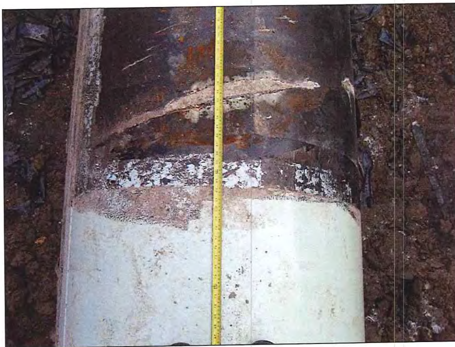
Photograph 9 • Site 1. Pipe Exposed. Corrosion at Overlaps.
