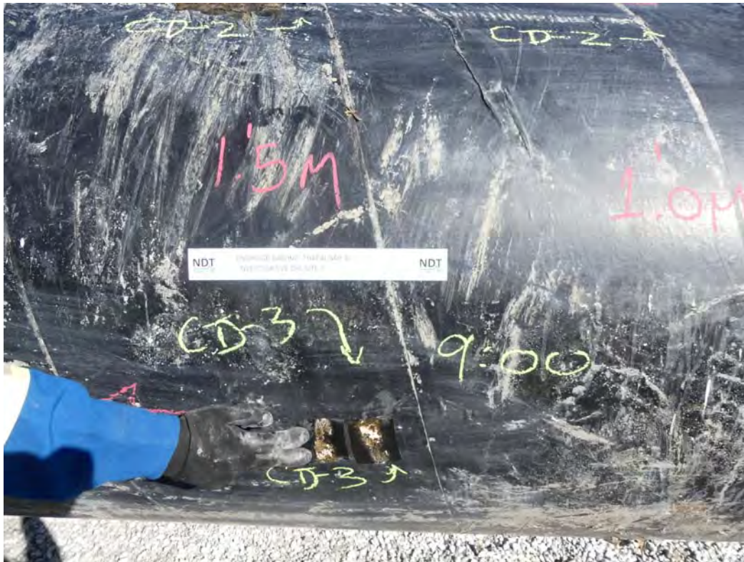
031 - CD-03 COATING REMOVED, CORROSION DEPOSIT AT 1.5 M
