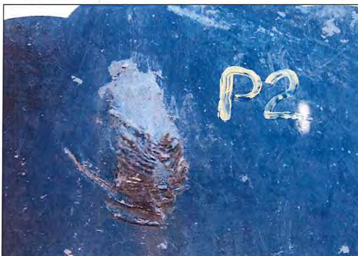
Photograph 5-22 • Site #2. Sample of Coating Damage by Locating Probe (P2)
