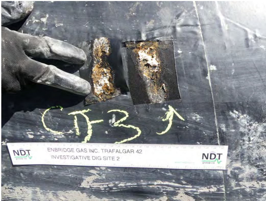
029 - CD-03 COATING REMOVED WHITE, BLACK CORROSION DEPOSIT (1)
