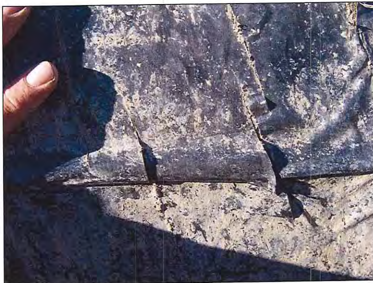
Photograph 5-20 • Site #2. Sample of Disbonded Coating along Longitudinal Weld. Close View
