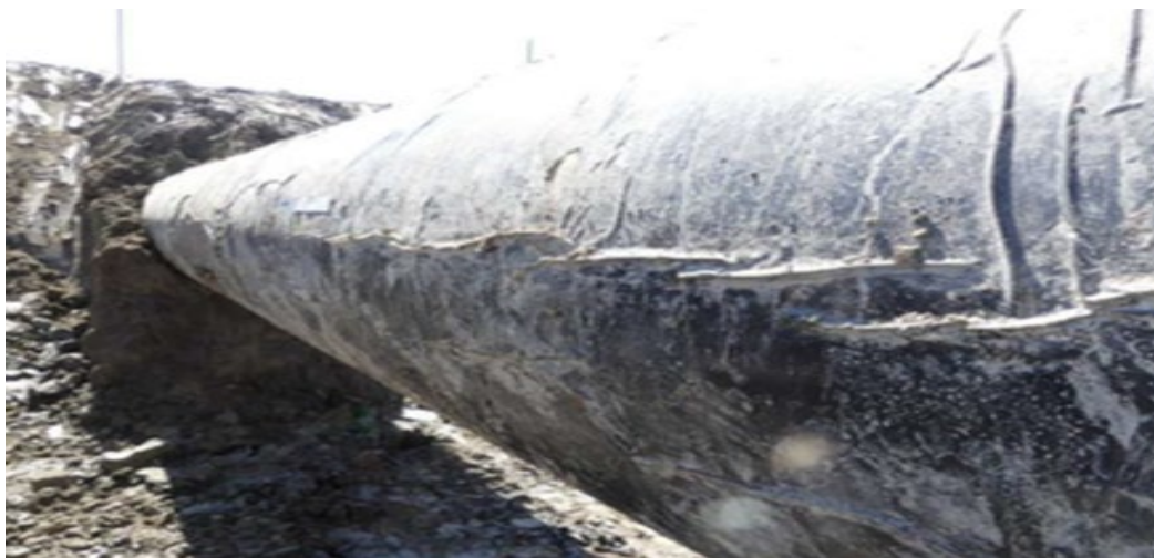
Figure 5: Typical Trafalger NPS 42 Dawn to Kirkwall Disbonded Polykin Tape
