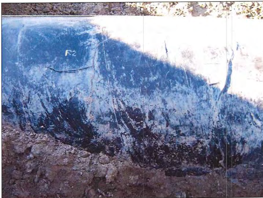
Photograph 9 • Site 2. Disbonded Coating at Longitudinal Weld. Looking North – 07.
