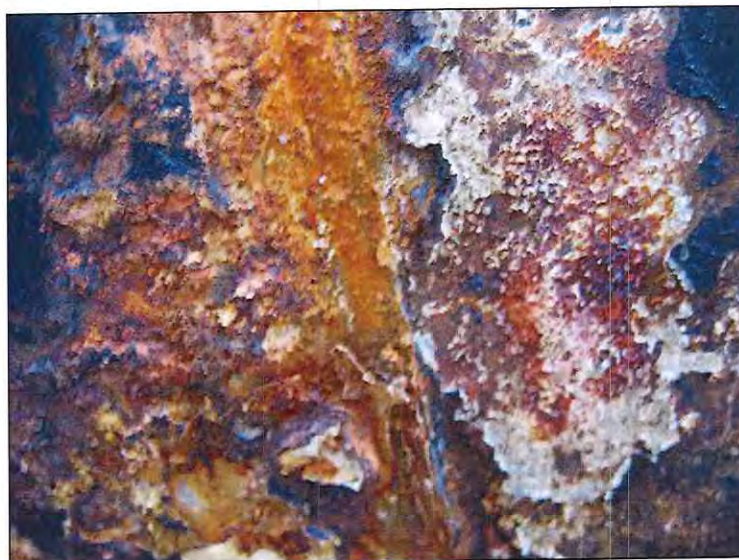
Photograph 5-8 • Site #1. Pipe Exposed. General Corrosion & Calcareous Deposits. Close View
