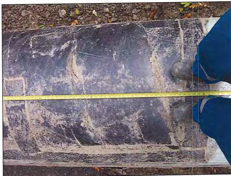
Photograph 5-5 • Site #1. Disbonded Coating at Overlap
