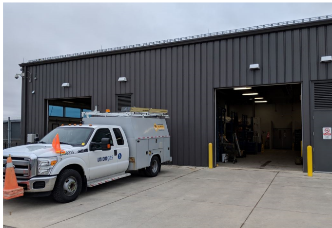
Truck Loading: Truck loading areas should be clear of obstructions and have bollards indicating exposed corners and doors. Areas should have adequate lighting.
