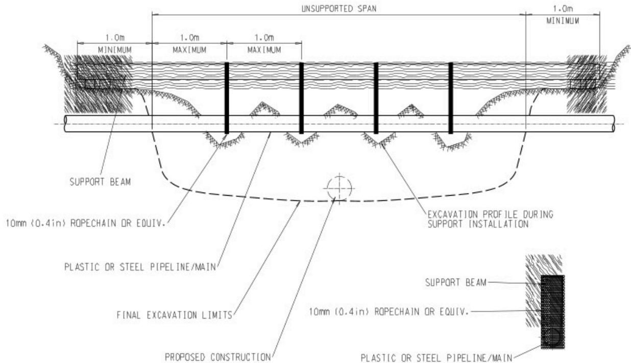
Figure 7-2: Typical Temporary Supports for Pipelines Crossing the Trench – Span Exceeds 4.5 m
