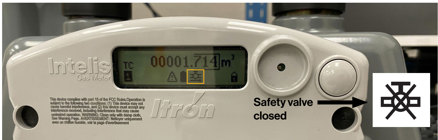
Image 2: Intelis meter showing safety valve indicator open and closed
