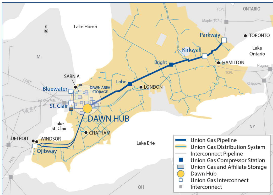
Figure 5.4.6.1.: Overview of Union’s storage and transmission system, showing major compressor plants
