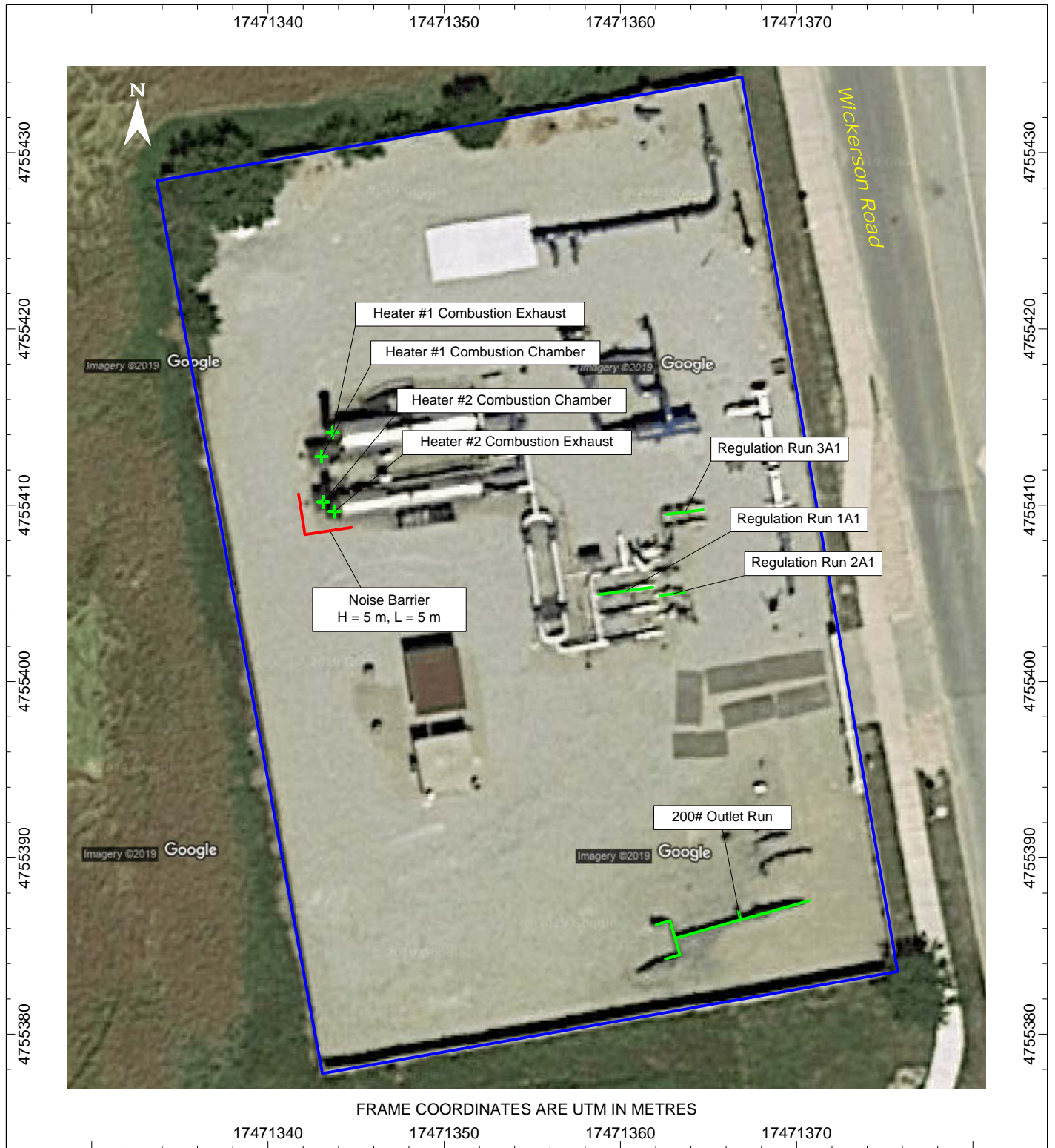
Figure 1: Union Gas Byron Transmission Station Showing Locations of Noise Sources and Potential Noise Barrier
